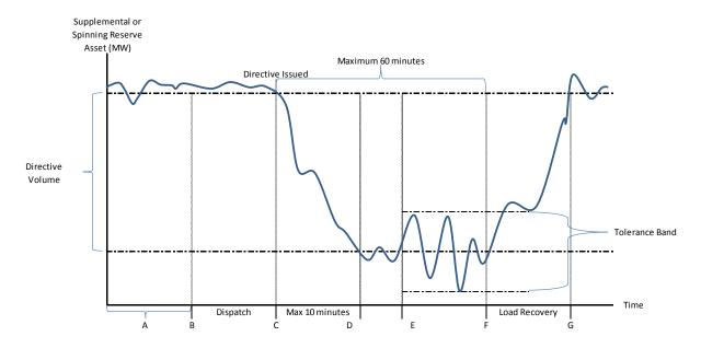
This figure illustrates a possible response from a load pool asset that is providing either spinning reserve or supplemental reserve. The meaning of the labeled points is as follows:
