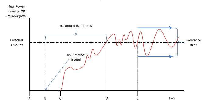
This figure shows a possible response from a generator that is not synchronized to the interconnected electric system providing supplemental reserve. The meaning of the labeled points is as follows:
