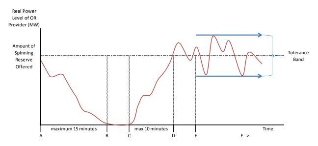
This figure illustrates a possible response from a pool asset that is synchronized to the interconnected electric system and is providing either spinning reserve or supplemental reserve. It is assumed that there are no energy market dispatches during the test time period. The meaning of the labeled points is as follows:
