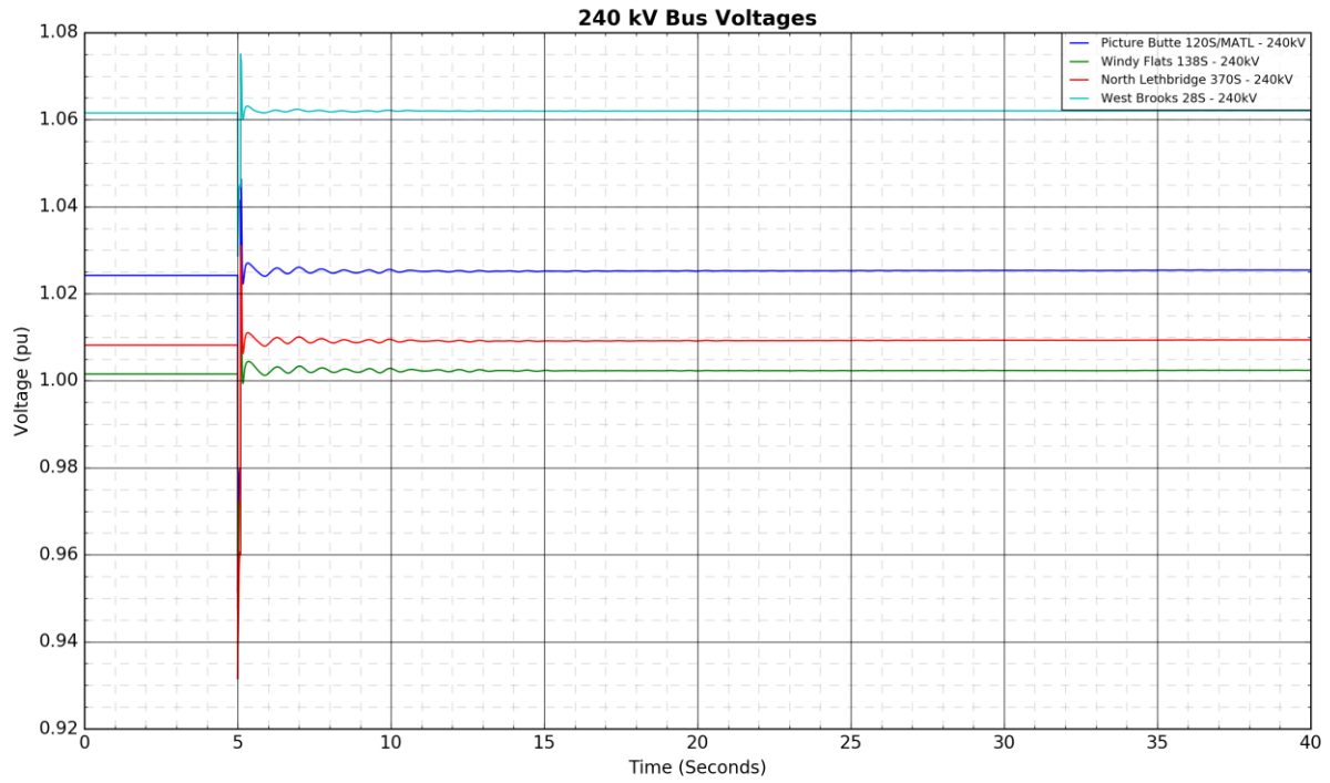
Figure A4-45: 225L Stirling 67S to Raymond Reservoir 313S T-Tap to Magrath 225S: Fault Near Stirling 67S
