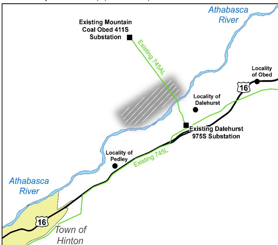
The black squares on the map indicate the approximate location of the existing Dalehurst 975S substation, which is at NW-21-52-23W5 and the existing Mountain Coal Obed 411S substation, which is located at NW-14-53-24W5. The grey shaded area on the map indicates the approximate location of the proposed transmission developments, including the 138 kV transmission line. The specific transmission facilities may extend beyond the grey shaded area shown.
