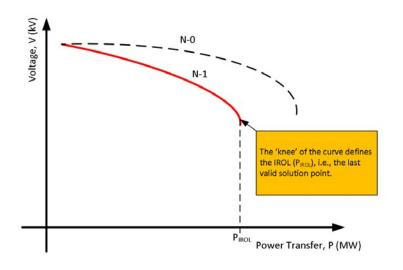
Figure 1: An IROL Example based on P-V Analysis:
