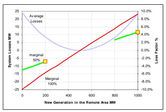
Figure 9: Marginal Loss Factor as proposed (with swing bus)
