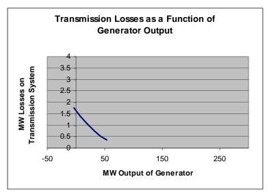
Figure 5: Scenario 2 MW losses on transmission system as a function of generator output.
