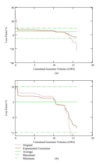
Figure 24 Impact of Exponential Correction Algorithm on Loss Factors
