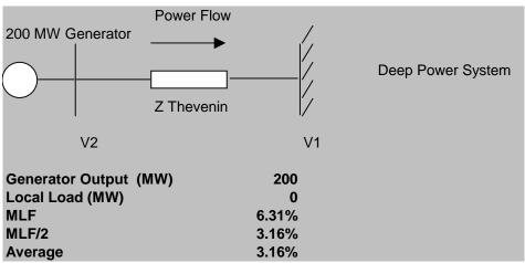
Figure 1: Scenario 1 Generator connected to an infinite bus through a radial transmission line.
