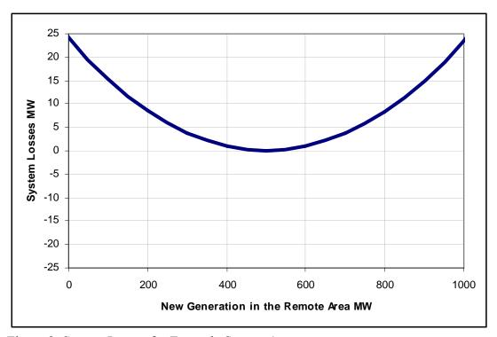
Figure 8: System Losses for Example System 1
