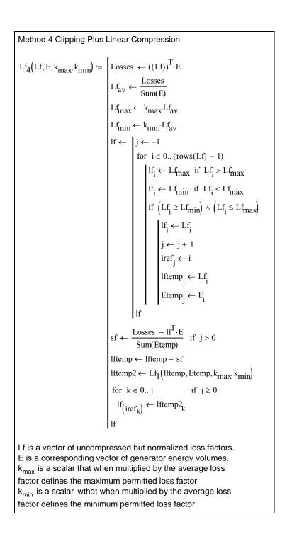
Figure 27 MathCAD Implementation of Clipping With Linear Compression Algorithm
