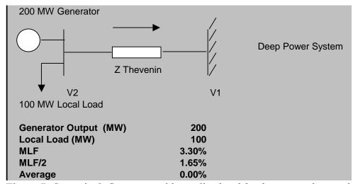
Figure 7: Scenario 3 Generator with smaller local load connected to an infinite bus through a radial transmission line.
