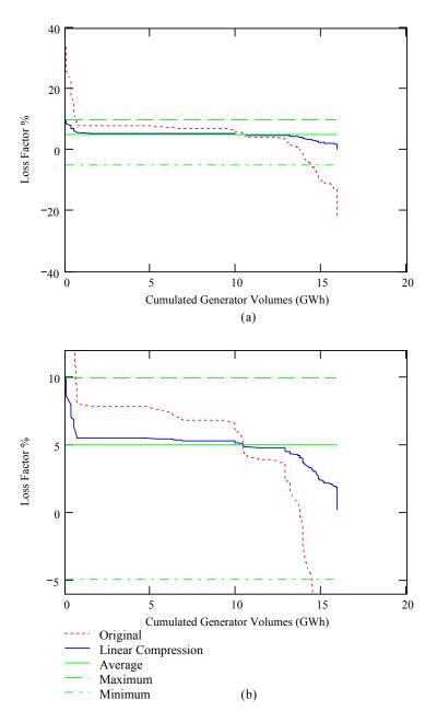
Figure 22 Impact of Linear Compression on Loss Factors
