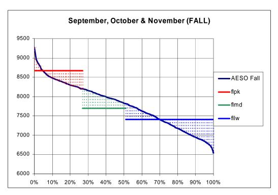
Figure 20 Weightings Based on Fall Load Flow Levels
