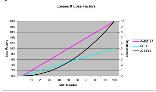
Fig 1: Losses Associated With a Flow Across Impedance
