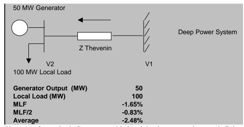
Figure 4: Scenario 2 Generator with local load connected to an infinite bus through a radial transmission line.
