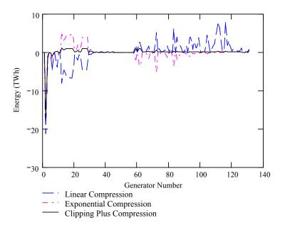
Figure 35 Changes in Individual Generator Loss Allocation Sensitivity to Smaller Magnitude Initial Loss Factors
