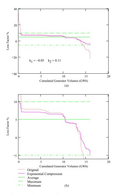
Figure 26 Impact of Exponential Compression Algorithm on Loss Factors
