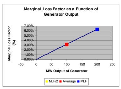
Figure 3: Scenario 1 Marginal loss factor as a function of generator output.
