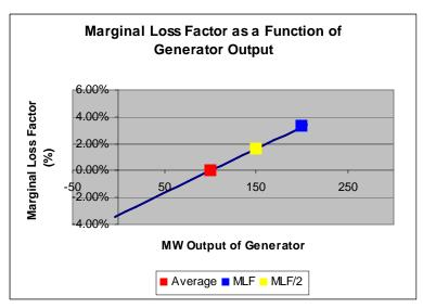
Figure 9: Scenario 3 Marginal loss factor as a function of generator output.
