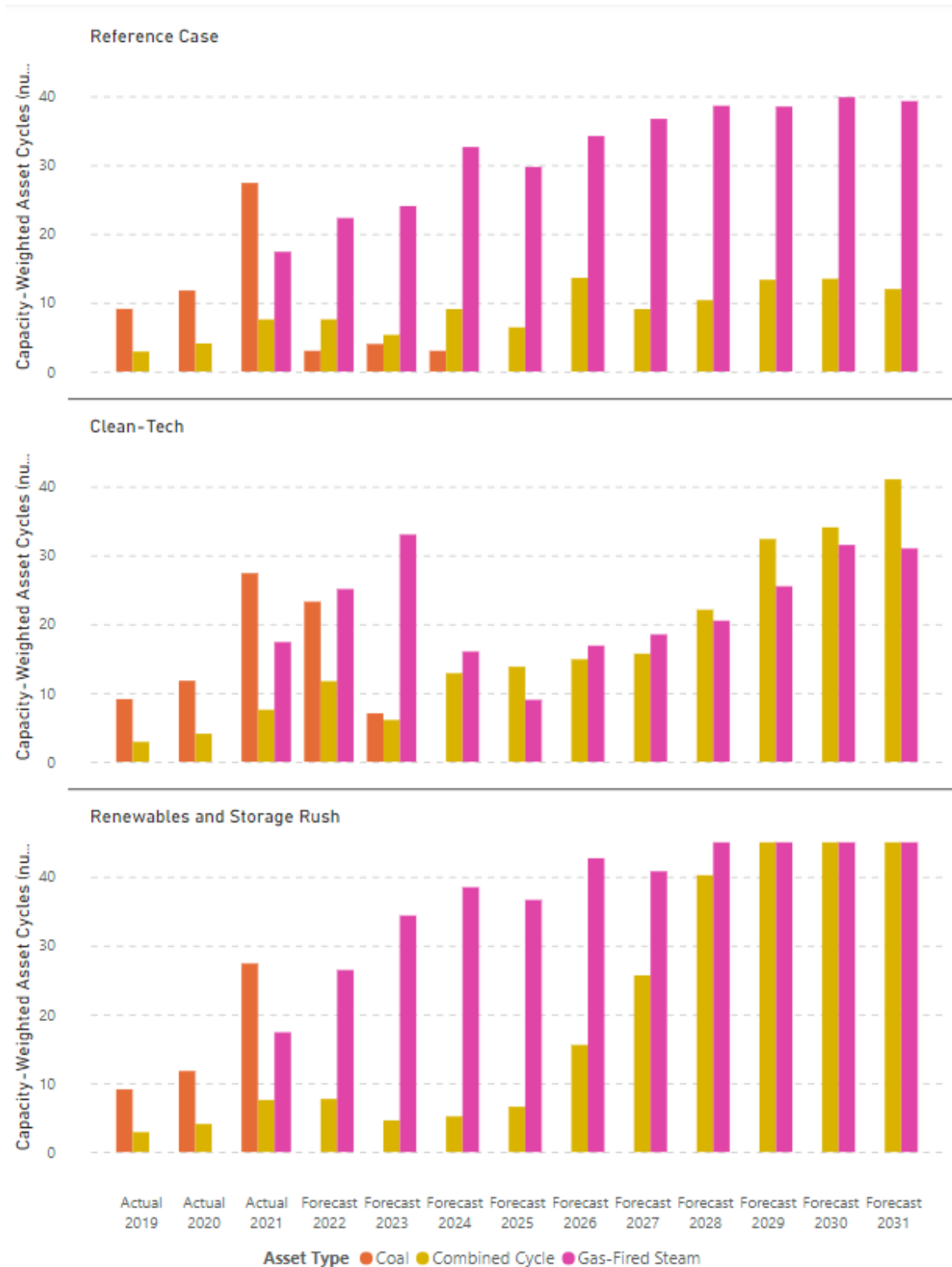
Figure 25: Average number of on/off cycles per generating asset by technology by scenario
